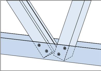
The diagonals should have contact in the joint. Use the amount of screws shown in the workshop drawing.
