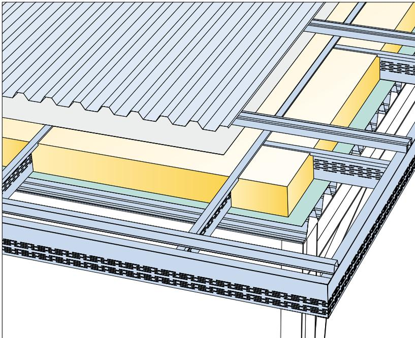
Lindab Thermo roof is a double skin roof which can use soft insulation. The roof build up is a floor deck profile (LTP 115 or LTP 150) in the bottom, vapour barrier, 150 or 200 mm slotted Z-profile, ZS, insulation, and on top of that a wind breaker hold in place by a secondary system (S7 45) and trapeze sheeting, LTP 20 or any other roof profile. Use DIMroof to design the floor deck profile hence the ZS-profile is just a distance there is no need for a static design for the ZS-profile. The
