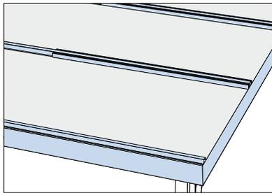
Use the Lindab hat profiles S7 45 as secondaries for the roof chosen roof profile.
