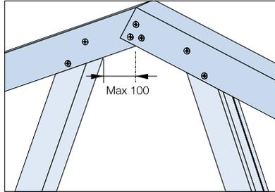
Top diagonal should end maximum 100 mm from the center of the top chord.
