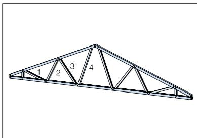
Mount the rest of the diagonals to fill up the frame. Make sure to mount the profiles with the open web upwards (back of the profile should be turned downwards)
