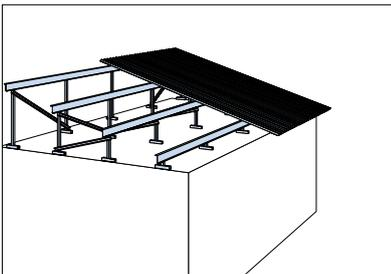
Cover the construction with the Lindab LTP20 or LTP45 roof.
