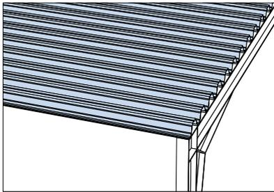
The underlay to build the thermo roof is a floor deck profile.
