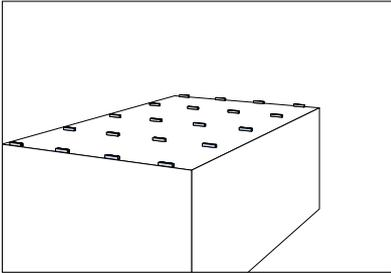
Mount the Lindab FSK60 base runners with fasteners approved for the underlay. Place them according to your dimensional drawing.
