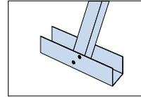
Place minimum two screws on each side.
