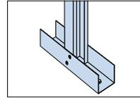
Place minimum two screws on each side.
