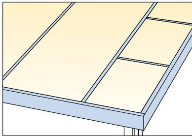
Fill up with insulation between the compartments. Important to use same insulation height as the height of the studs.
