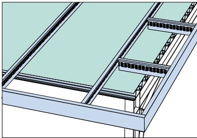
Build up the frame with slotted Lindab SZ-studs. Optional as shown in picture its possible to build with a roof overhang.
