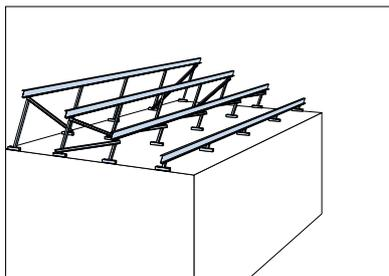
Make sure to stabilise the construction with cross bracings.
