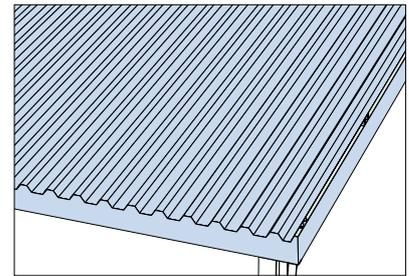
Assemble the roof profile on top, and cover with flashings.
