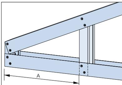
Place the first perpendicular diagonal at a distance from the gable according to the workshop drawing.
