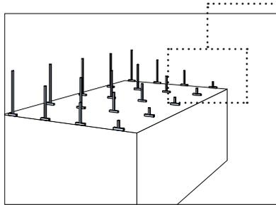
Fasten the Lindab FR studs on the runners in vertical position.
