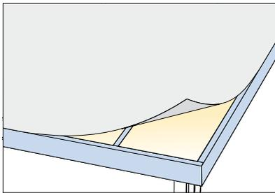
A wind breaker is placed on top of the insulation.
