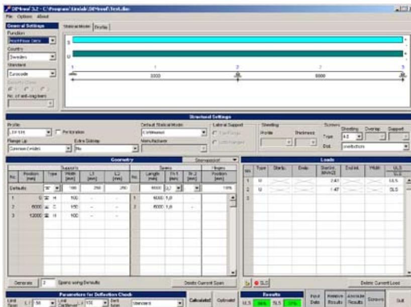
DIMroof can be used to analyze static design of different purlin systems. Overlap systems, simply supported and more advanced variants can be analyzed.
