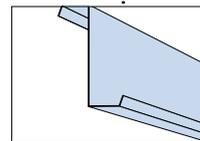
A standard Z-purlin can be used thanks to the leaning stud. The flange will be perpendicular to the roof cover.
