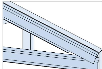
Gable trusses can have battens assembled along the frame before installing.
