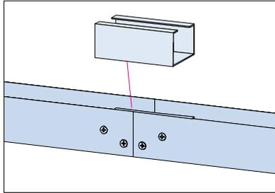
For larger spans the runners are split into half – the joint is done by using a short stud which will fit into the runners. Join them together with screws according to the workshop drawing.
