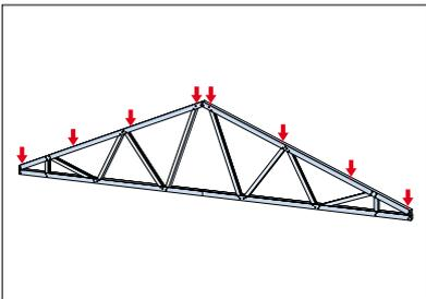
Mark out the battens before installing the roof truss on site.
