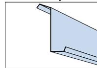
The customised Z-purlin is designed with a flange according to the roof pitch.
