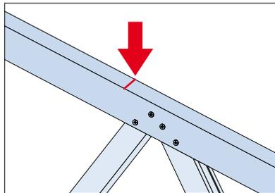
Battens should be placed close to the joints to transfer the loads optimal.
