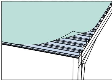
Place a vapour barrier on top of the deck profile.
